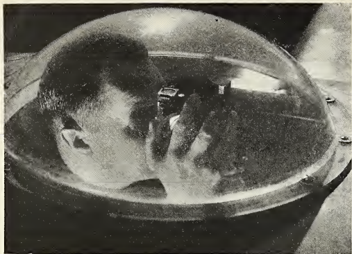
Proper position for the head and sextant in the spherical astro-dome is demonstrated (left) by Colonel Thurlow. This position allows for a minimum of refraction error. At right is shown the correct position as viewed from inside the plane.
